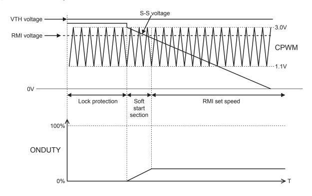
Adjust the S-S pin voltage gradient by means of the capacitance of the capacitor between the S-S pin and 5VREG. Recommended capacitor:  $0.1\mu$  to  $1\mu$ F
